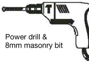
Power drill & 8mm masonry bit
