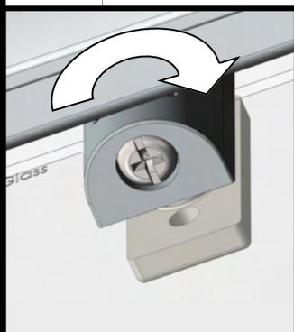
Turn adjusting screws clockwise to raise door. Adjust height & angle until doors run smoothly, magnets are parallel & hold doors closed with no gaps. Check that bottom wheels are engaged securely in bottom track (adjust upward until no wobble in bottom track).
