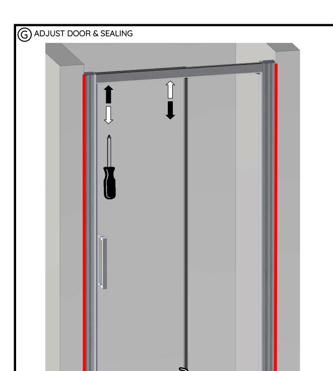
From underside of top wheels, adjust door height until bottom wheels are engaged in horizontal profile (no wobble). Then adjust door angle plumb with vertical frame profiles (check door edge contact with bump stop).
