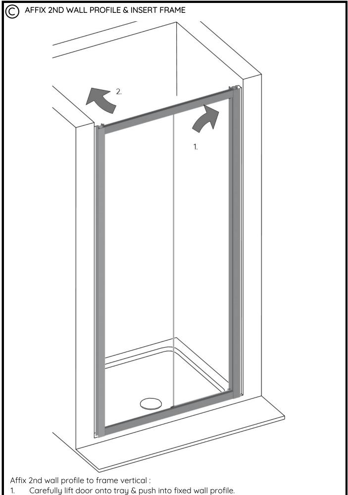
At loose side, push back, re-align & affix wall profile to wall using 4 x 45 long screws.
