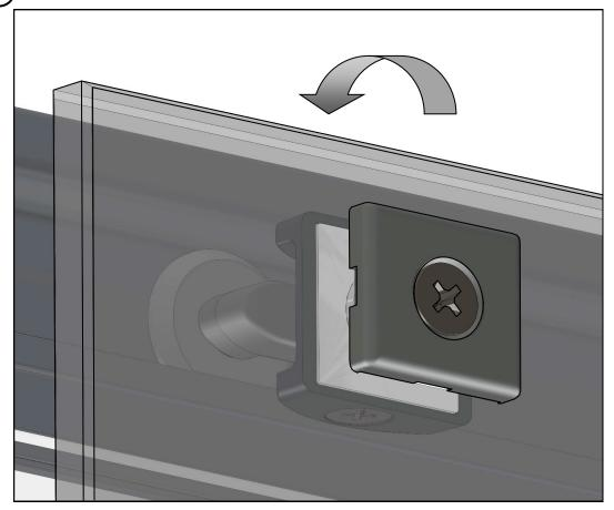
Carefully lift door into enclosure & engage top wheels into wheel groove. (If necessary loosen, but do not remove centre screw to permit engagement). Immediately after wheels are correctly engaged, fully tighten centre screw to retain door. Fit internal wheel covers \*\*.
