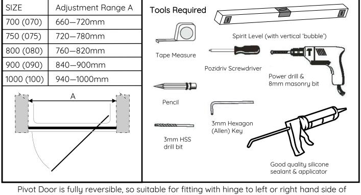
Pivot Door is fully reversible, so suitable for fitting with hinge to left or right hand side of enclosure. Ensure tray is correctly levelled & that all tray/wall joints are sealed & cured over entire length of tray sides (See – – – – – Fig A) prior to fitting enclosure. DO NOT SEAL BASE / WALL EDGES UPTO A FITTED ENCLOSURE !
