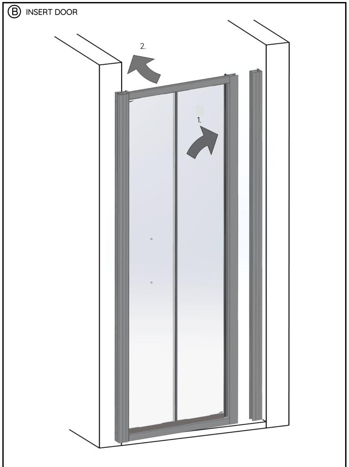
With 2nd wall profile fitted to frame:
