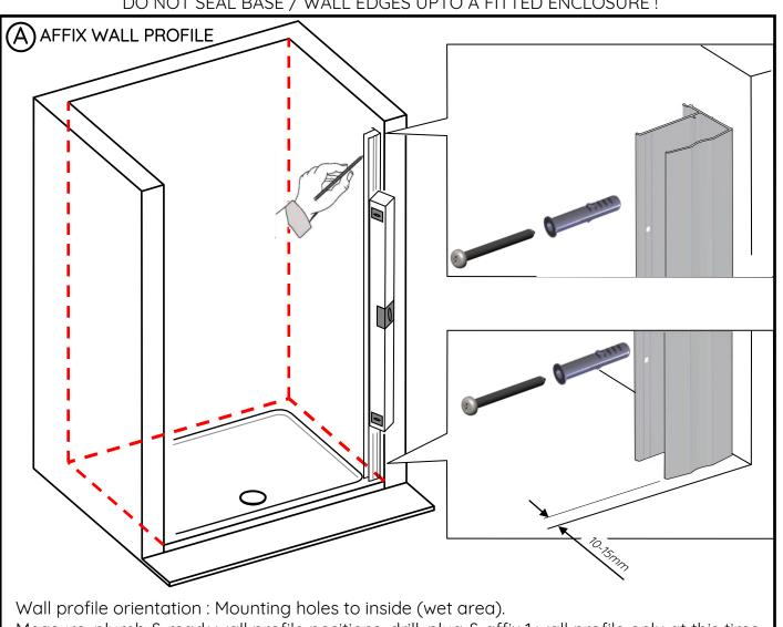
Measure, plumb & mark wall profile positions, drill, plug & affix 1 wall profile only at this time.
