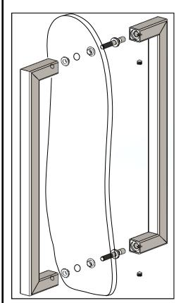
Assemble handle to glass as shown (grubscrews to inside). Ensure plastic fitted each washers are side beneath handles. Tighten grubscrews fully to retain.
