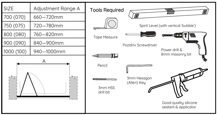
Pivot Door is fully reversible, so suitable for fitting with hinge to left or right hand side of enclosure. Ensure tray is correctly levelled & that all tray/wall joints are sealed & cured over entire length of tray sides (See - - - - Fig A) prior to fitting enclosure. DO NOT SEAL BASE / WALL EDGES UPTO A FITTED ENCLOSURE!
