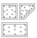
With your shower tray upside down, position all (DO NOT PERMANENTLY FIX AT THIS STAGE) the leg assemblies to form an evenly supported structure. Wherever possible use the full number of leg assemblies available for maximum support.
