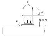
Attach the Panel Upright Brackets ③ using two screws ③ to the Circular Base Plate assemblies ⑤ that are located on the panel access sides of the tray.
