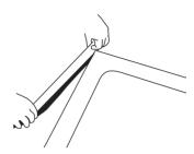
Wipe the surfaces clean where the strip will be attached first with a clean damp cloth, allow to dry and then wipe with the IPA wipe supplied in the kit.
