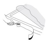
Note! Some shower trays have a protective film (indicated by a label on the surface) which must now be removed. Undertake a final inspection of the shower try at this stage. DO NOT PROCEED IF NOT SATISFIED.
