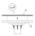
Attach the Circular Adhesive Pads **(3)** to the under-side of all the Circular Base Plates **(9)** by removing the backing paper from one side ONLY of the Adhesive Pads **(3)**, centralise and push firmly into position.
