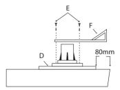
Attach the Panel Upright Brackets ( using two screws ( to the Circular Base Plate assemblies ( that are located on the panel access sides of the tray.
