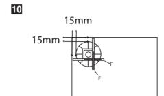
Once an evenly supported layout plan has been achieved, ensure the base of the tray is clean and free from dust and other contaminates, then remove the remaining backing paper from the Adhesive Pads ① on the leg assemblies ① and attach all the assemblies permanently into position.
