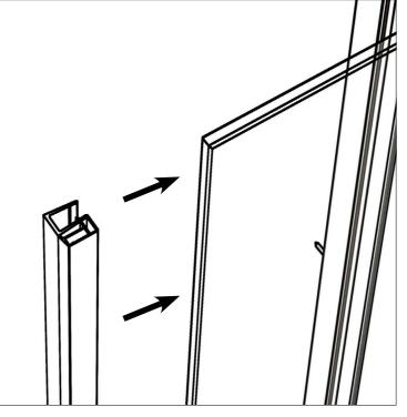
Step 7: ENSURE SEAL IS FITTED TO BASE OF DOOR. IF REQUIRED, REMOVE SEAL AND FIT TO BASE FOLLOWING INSTRUCTIONS BELOW:
