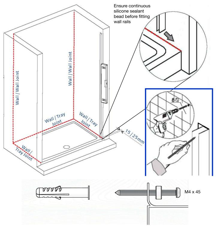
Step 1: Measure & mark wall rail positions. Mark fixing hole positions, drill & plug walls.
