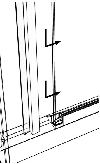
Step 6: Fit magnetic seal so ends are flush with glass top and bottom. Ensure magnet is fitted on internal side.
