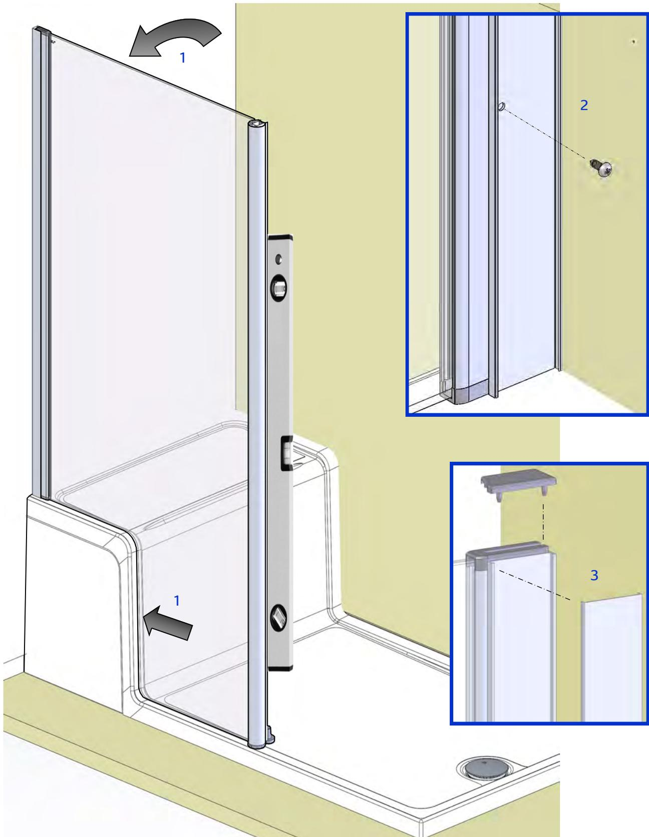
2. With panel positioned and plumb, from inside enclosure, using wall profile holes as a guide, drill dia 3mm & affix panel to wall profile using 3.5 x 10 pan head screws (3 places).
