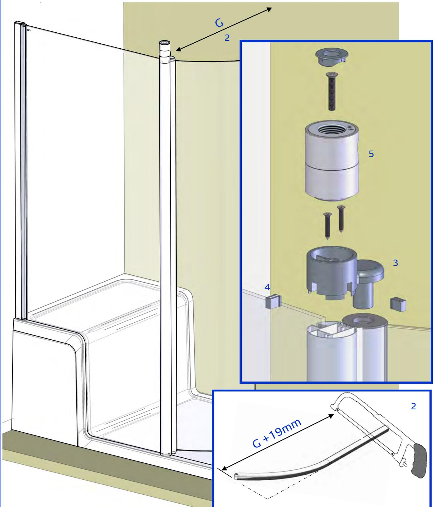
2. Fit door assy onto bottom hinge. Keeping the door supported, push fully down & back onto the hinge seals, then assemble top hinge bracket (joining door to post profile). Immediately affix with 2x 4 x 25 long CSK self tapping screws.
