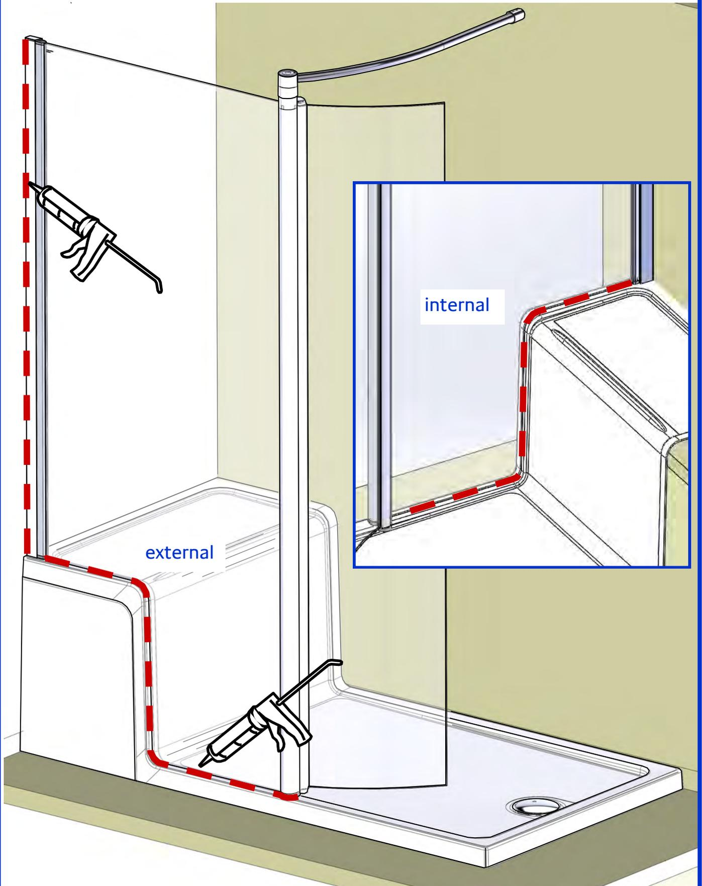
Use of good quality silicone sealant & cleaning / degreasing of all joint areas is recommended. Apply continuous silicone sealant beads as indicated. For glass to tray joint lines, the use of silicone to both sides of glass, & using silicone shaping tool is recommended to achieve sealing & best appearance.
