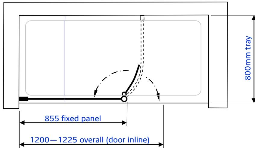
Walk In Enclosure is fully reversible, so is suitable for fitting to left or right hand wall. Ensure tray is correctly levelled & that tray / wall (tile) joints are sealed & cured over entire length of tray sides (See Fig A) prior to fitting enclosure.
