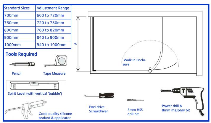
Lakes Walk In Return Panel is fully reversible, for use in conjunction with, & fitting to left or right hand Walk In Enclosure. Ensure tray is correctly levelled & that tray / wall (tile) joints are sealed & cured over entire length of tray sides (See Fig A) prior to fitting enclosure.
